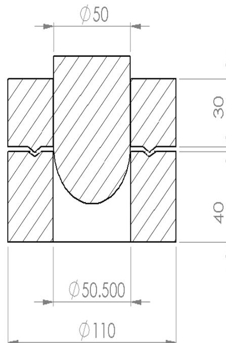
**Fig 3.1** Schematic diagram of the tools used in stretch forming experiments
