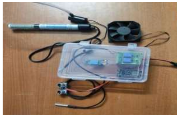
Fig.7.1 Hardware setup of Smart fish tank
