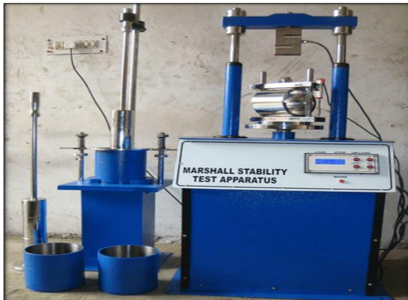
Figure 3.1 Marshall Stability Test Apparatus.
