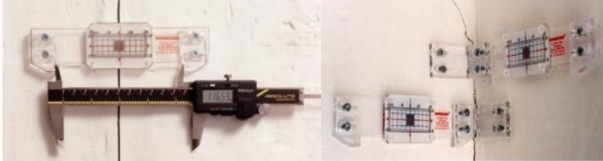
Figure 3: Crack Monitoring Equipment
