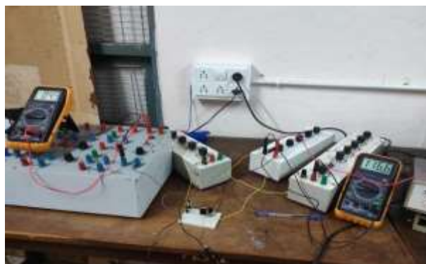
Fig 3: Conduction of Basic Booster Hardware circuit
