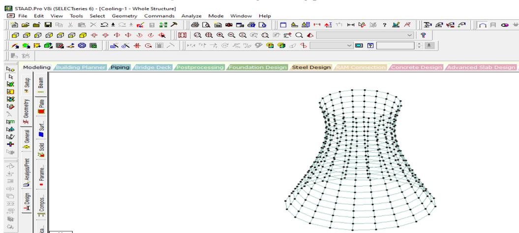
Figure 2: Geometry of the cooling tower
