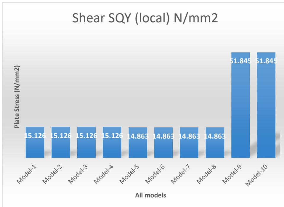
Figure 5: Shear stress (SQY) for all the models
