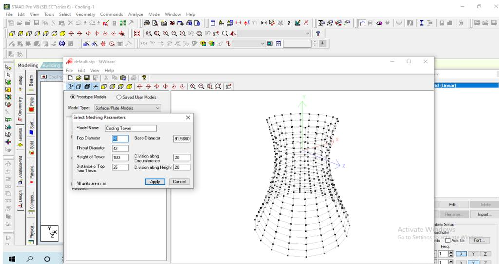
Figure 1: Selecting meshing parameters
