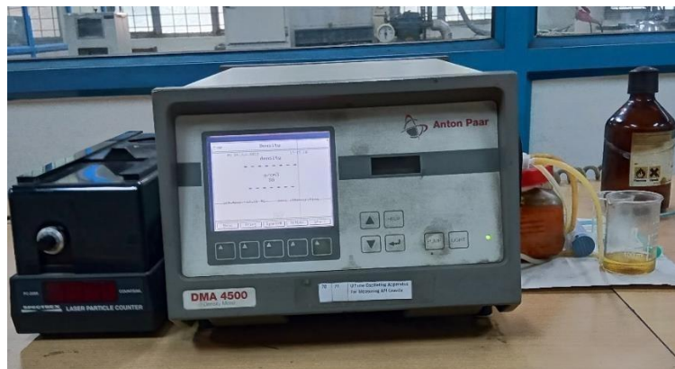
fig.3: Instrument used to determine the density
