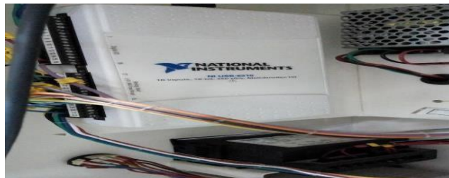
fig.5: Test engine set-up: NI Data acquisition system
