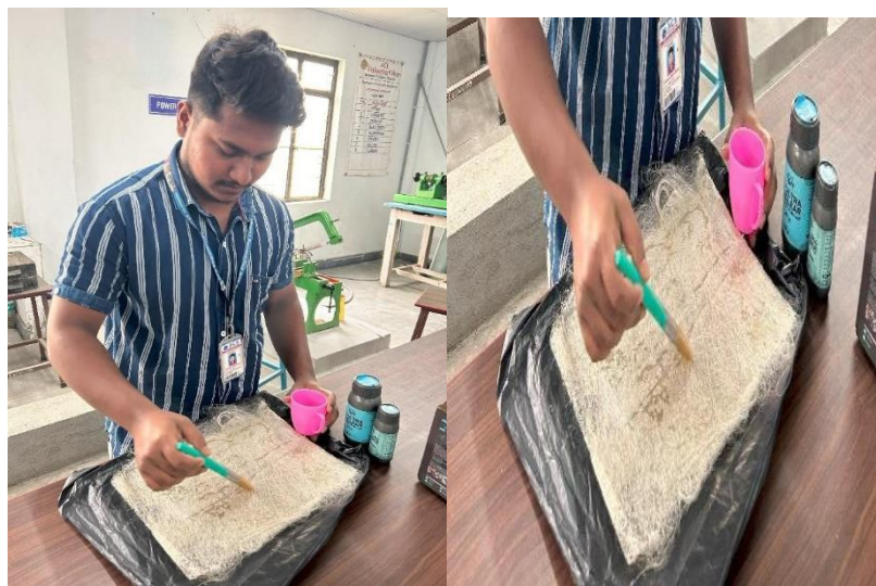
Fig: 4.2 Applying resin to cocoon matrix
