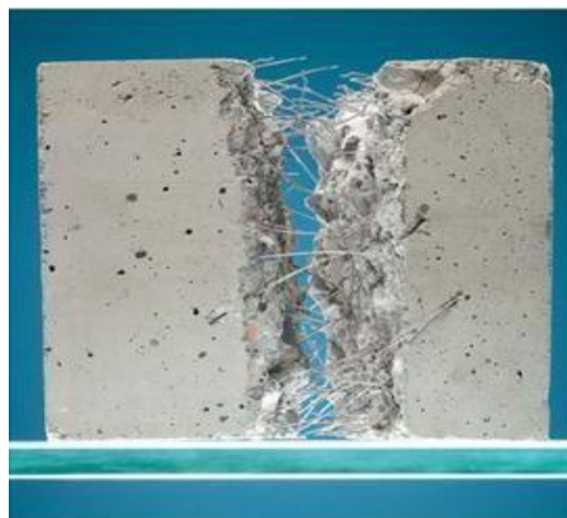
Figure 1.1 Steel fiber in concrete
