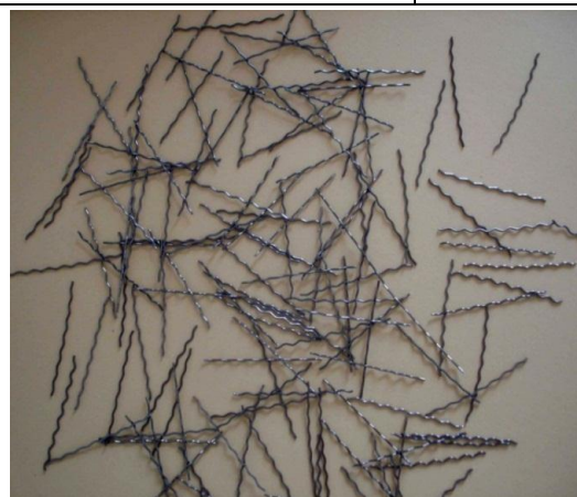
Figure 4.3 Corrugated type steel fiber
