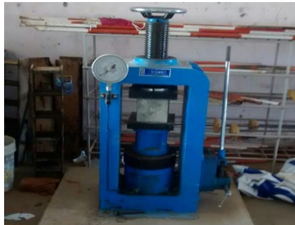
Figure 5.1 Compression test on cube specimen
