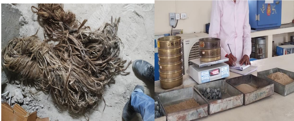
Figure 4 Process of preparation of stone column by clay soil, jute geotextile and stone chips
