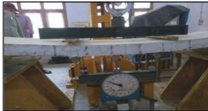
Fig. 4: Test set up for Static loading under loading condition
