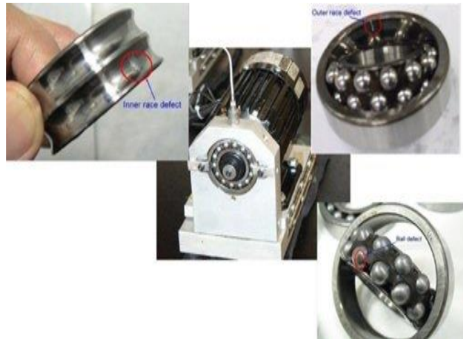
Figure 3 The Motor Bearing Fault
