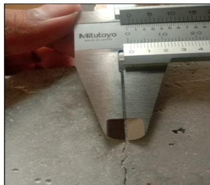
Fig 5.10 Measurement of cracks using Vernier Callipers
