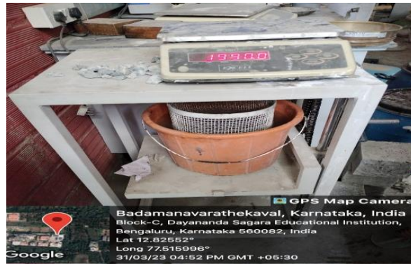
Fig.3.7 Specific gravity test of Coarse aggregate
