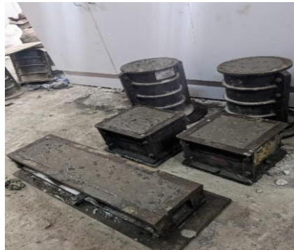
Fig: 3.8 Placing of concrete in the moulds
