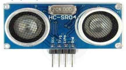
The HC-SR04 Ultrasonic sensor commonly known as Ultrasonic distance detector is a sensor which has two transducers which are Ultrasonic. Among the two transducers one acts as a transmitter and the other acts as a receiver. The sensor which can convert an ultrasonic signal into an electrical signal or energy signal is known as an Ultrasonic sensor
