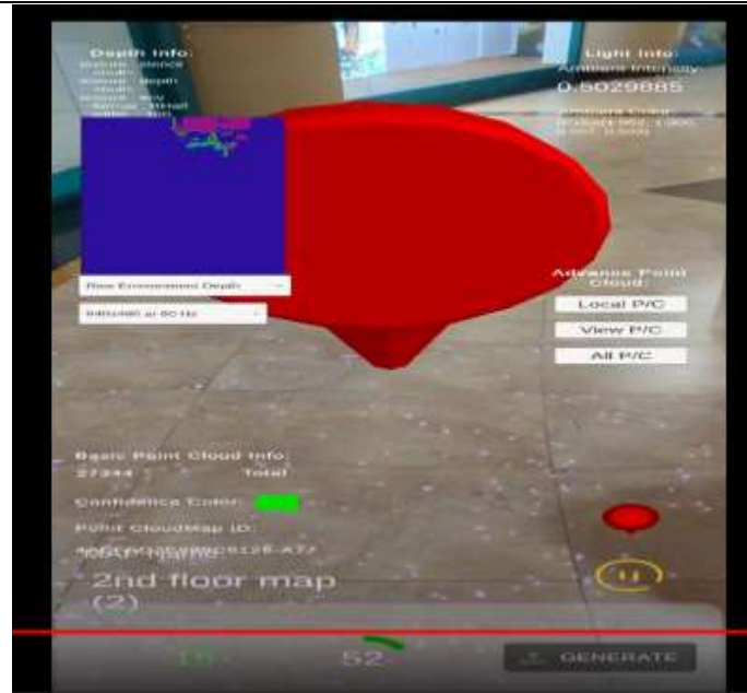
Fig.9. Creating destinations within mall so user can select desired destinations. Generation of point cloud data for creating the same.
