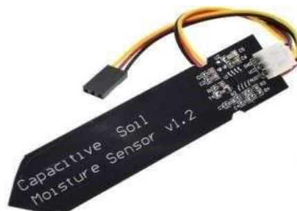
Figure 6 Capacitive Soil Moisture Sensor
