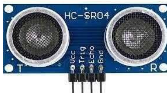
Figure 2: Ultrasonic Sensor (HC-SR04)
