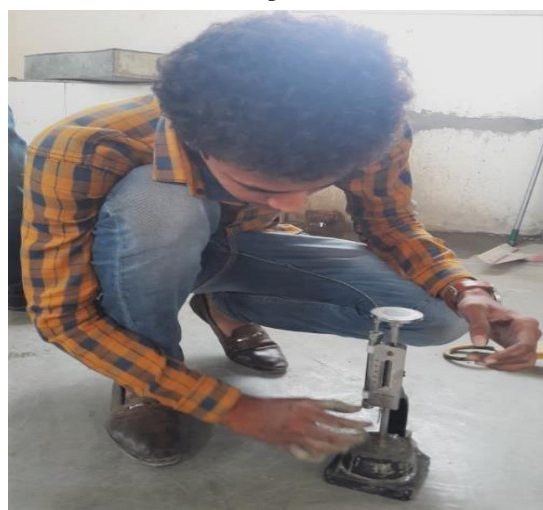
Figure. 4.2 Vicate apparatus for consistency of cement alculatation:
