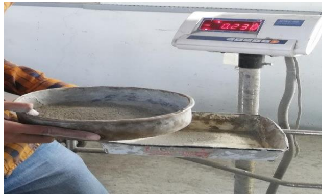
Figure 4.1 Fineness of cement
