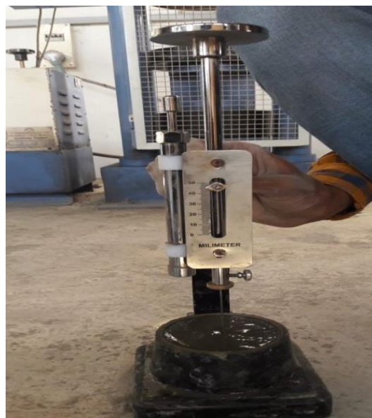
Figure. 4.3 Vicate apparatus and Glass plate for initial and final setting time
