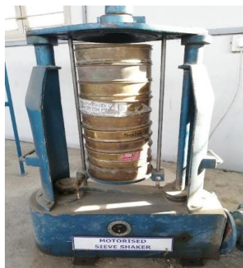
Figure 4.5 Sieve shaker for fine aggregate
