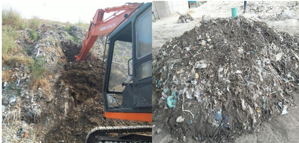
Figure 4.2 (a) Excavation of MSW Sample (b) Air drying of sample on site
