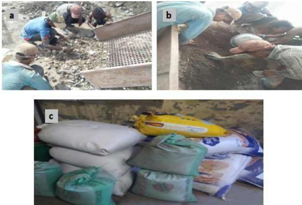
Figure 4.4 (a) Manual screening of SMSW (b) Sieving through 4.75 mm sieve (c) Collected SMSW sample
