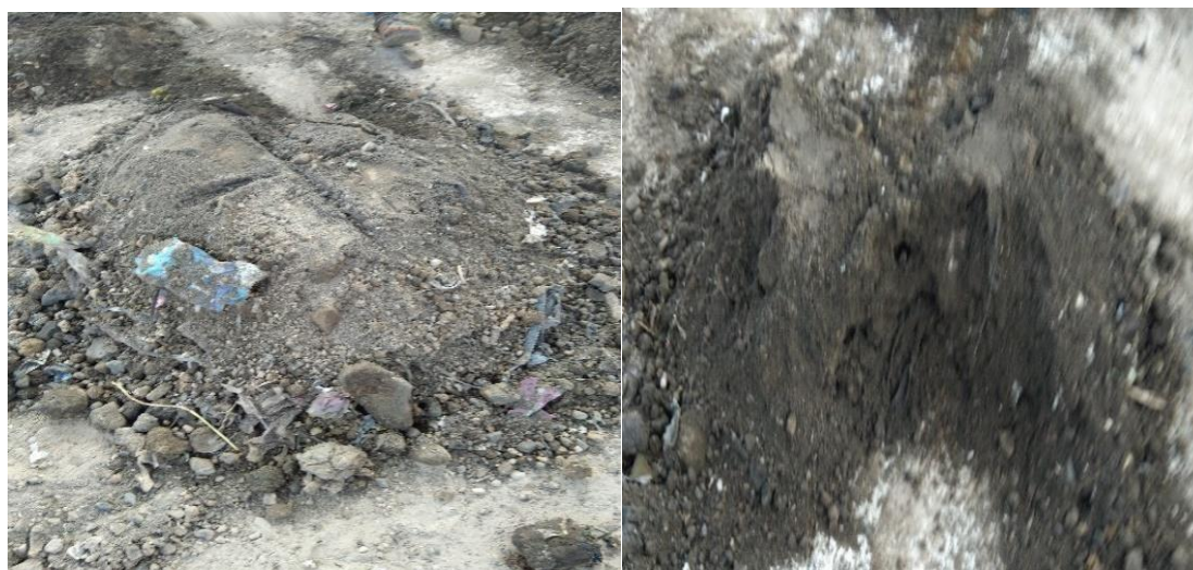
Figure 4.3 Coning and quartering technique (a) The divided four parts (b) Retained two parts
