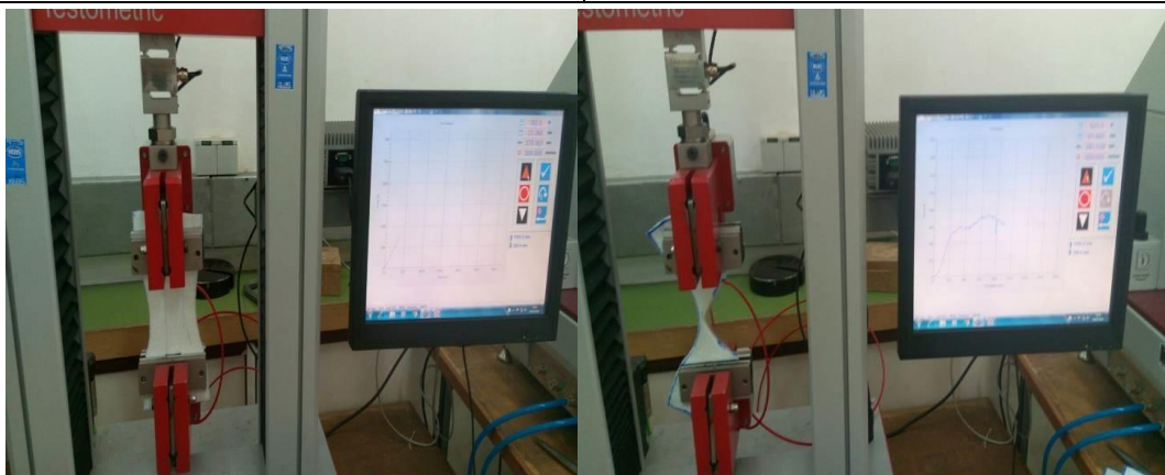
Plate 4.1: Grab Strength Testing Plate 4.2: Trapezoidal Tear test
