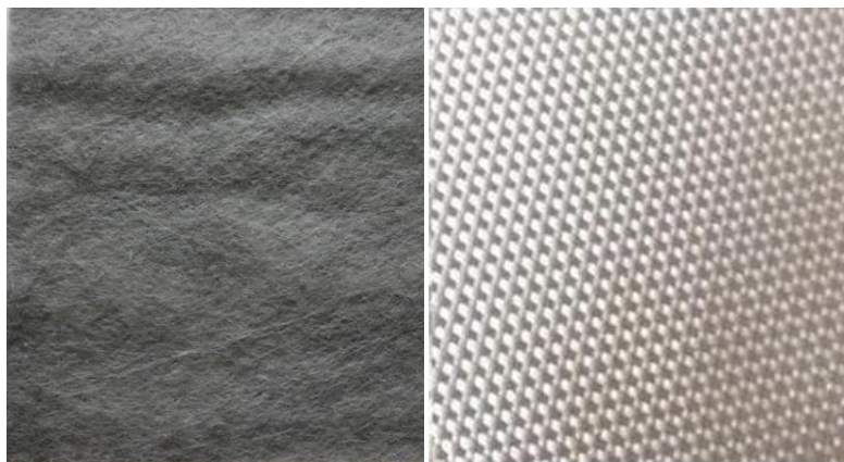
Plate 1.1: Geotextile made of non-woven material (Author 2017 as the source) Plate 1.2: Woven geotextile (Author, 2017 is the source for this phrase)
