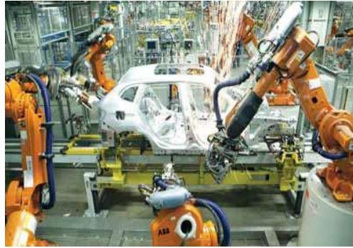
Fig. 15 Riveting an automobile frame using a robotic arm.
