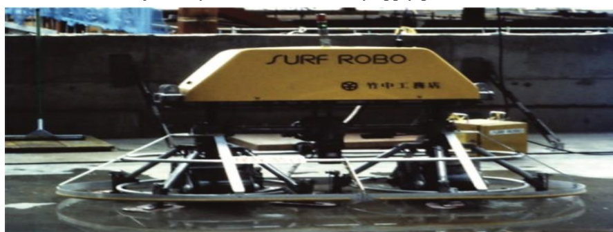
Fig. 23 Surf Robo concrete finishing robot
