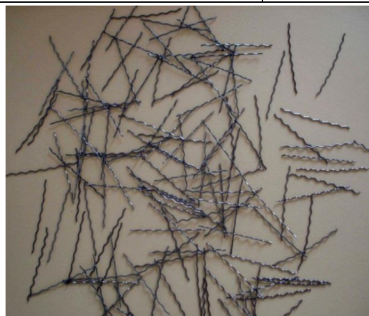
Figure 4.3 Corrugated type steel fiber
