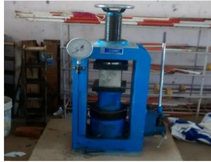
Figure 5.1 Compression test on cube specimen
