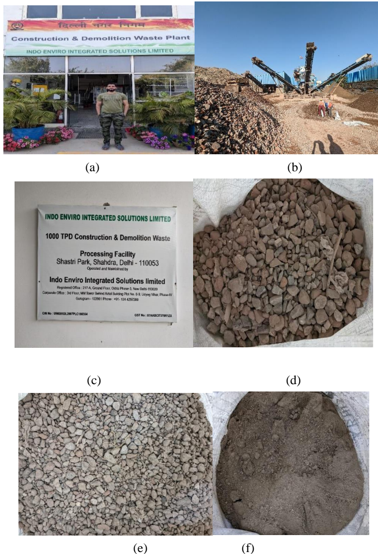
Fig. 4.2. (a) C&D demolition waste facility; (b) Crushing & Segregation unit; (c) C&D unit details; (d) 20mm CRCA sample; (e) 10mm CRCA sample; (f) FRCA
