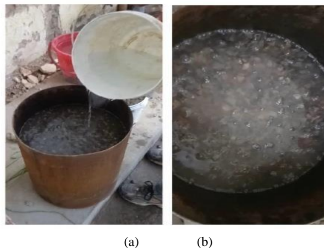
Fig. 5.1 Using a mild acid to treat CRCA.
