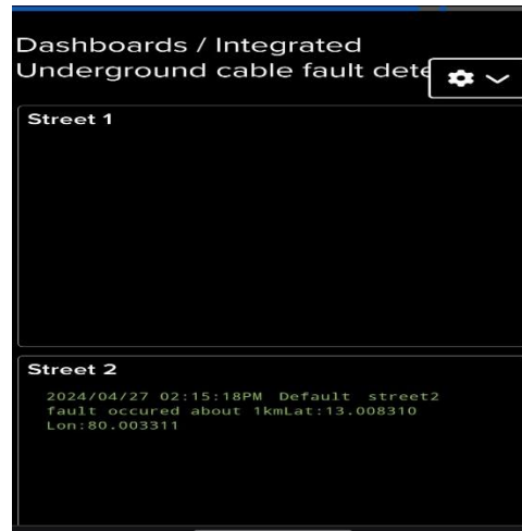
Fig 10. GPS location of fault occurred area fetched via cloud.
