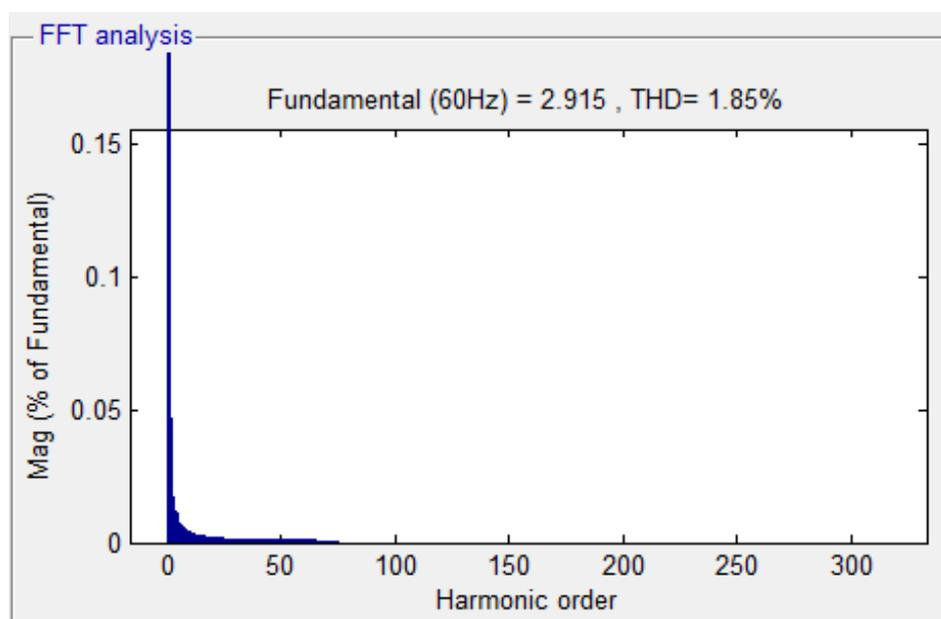
**Harmonic order A Combination of Shunt Hybrid Power Filter and Thyristor-Controlled Reactor in dynamic state condition**
