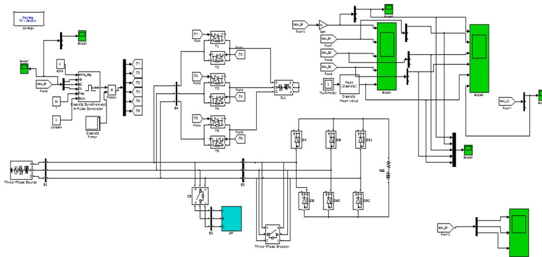
circuit configuration of A Combination of Shunt Hybrid Power Filter and Thyristor-Controlled Reactor in dynamic state condition
