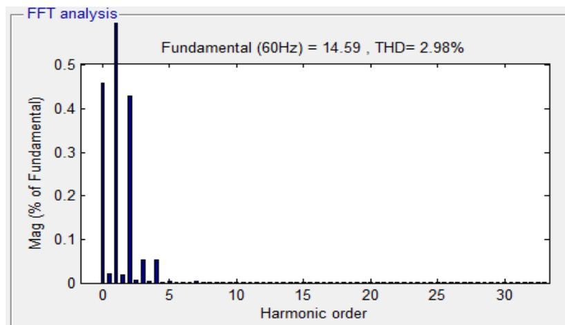
Harmonic order A Combination of Shunt Hybrid Power Filter and Thyristor-Controlled Reactor in steady state condition
