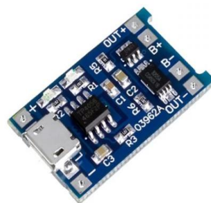
Figure 2: Lithium Battery Management System
