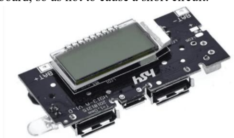
Figure 4: Power bank charging module with digital display
