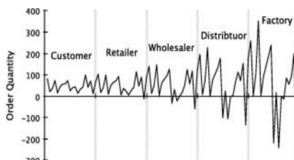
Fig3.1: A simple example of the Bullwhip effect
