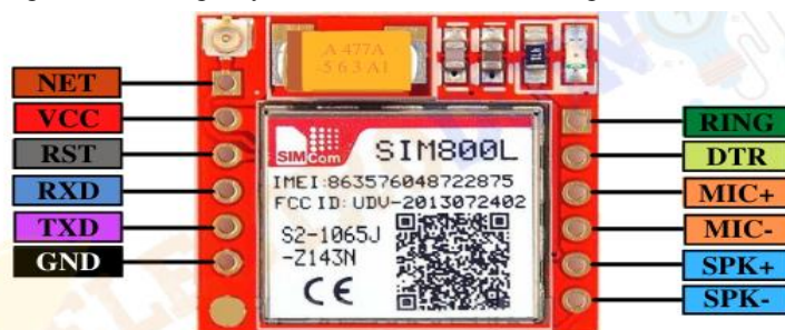
Figure-5 shows SIM800 pinout
