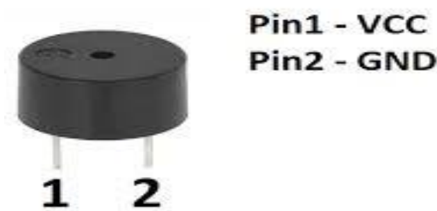
Figure-6 shows the pinout of Buzzer.
