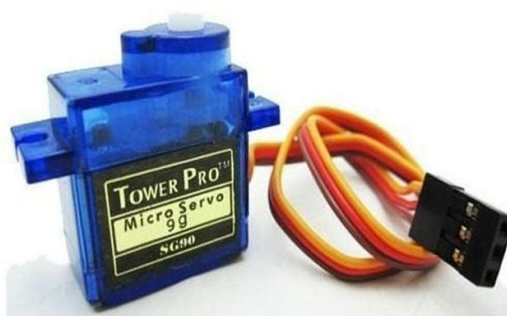
Figure-4 shows servo motor
