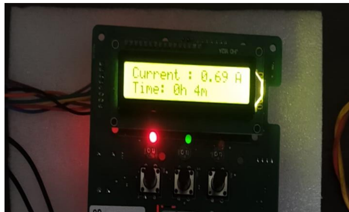
Figure4: image of current measuring of load
