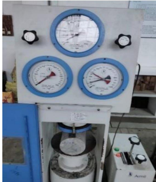
FIG 2 : CYLINDER UNDER SPLIT TENSILE STRENGTHING MACHINE
