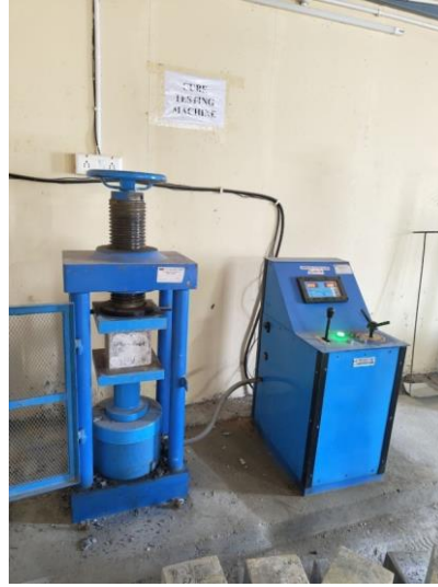
Fig 1 : CUBE UNDER COMPRESSION TESTING MACHINE
