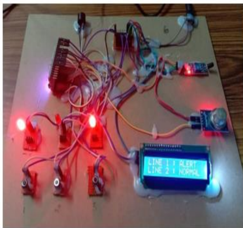
Figure 14: Cable 1 and Cable 3 Fault Condition
