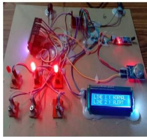
Figure 15: Cable 2 and Cable 3 Fault Condition
