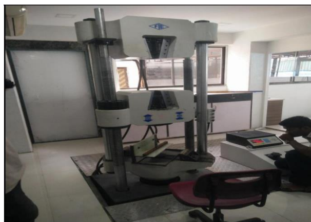
Figure .1 Test setup for battery bracket
