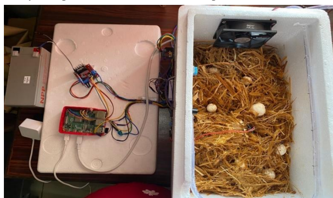
Figure 4: Setup of the IOT mushroom farming
