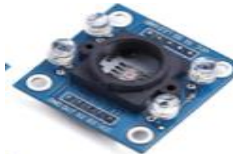
Fig 2: TCS3200 Colour sensor
