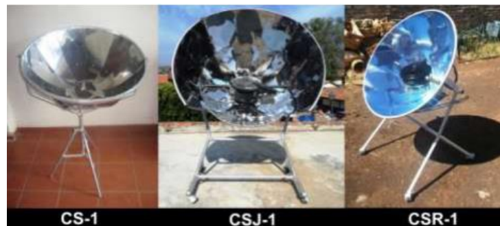
Figure 2: Solar Cookers CPC of revolution
