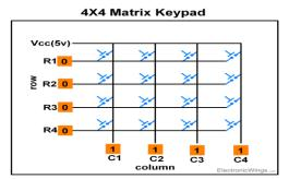
4x4 Keypad PinoutThe columns and rows make up the matrix layout of the keyboards. The columns and rows make intimate contact if a key is pushed. If not, then rows and columns don't have any significance.
