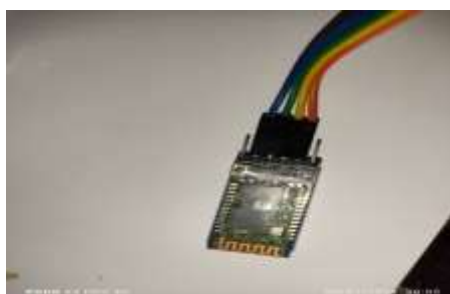
Figure 5.3 Hc05 Bluetooth Module
