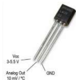
Figure 2- Temperature sensor (lm35)
