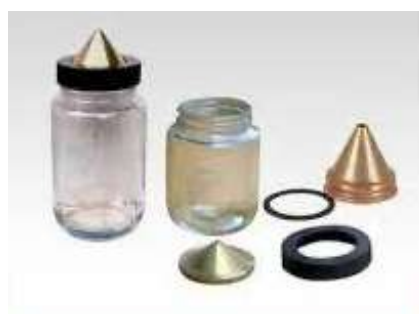
Figure. 2 Pycnometer used in laboratory
