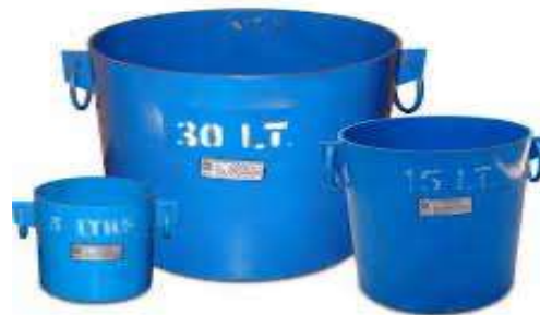
Fig.4 Cylinder used in laboratory for measuring density of aggregates.
