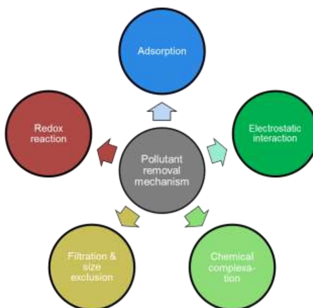
Figure 2: Mechanism involved in removal of pollutants from water by clay based nanocomposites
