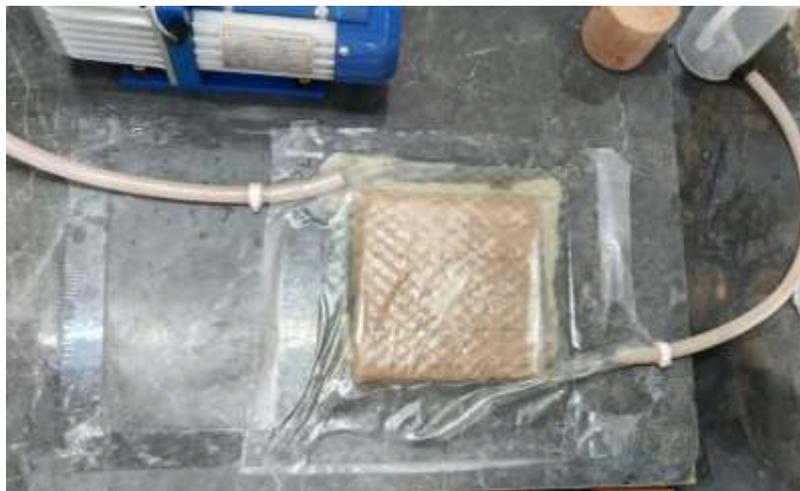
**Figure 3.** Lamination sequence followed to fabricate the composite laminate
