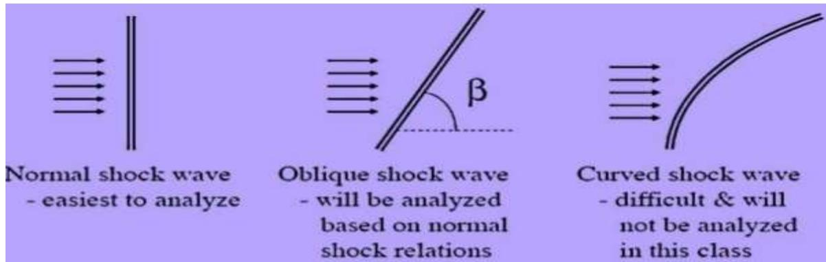
Fig.1.3: Types of shock waves
