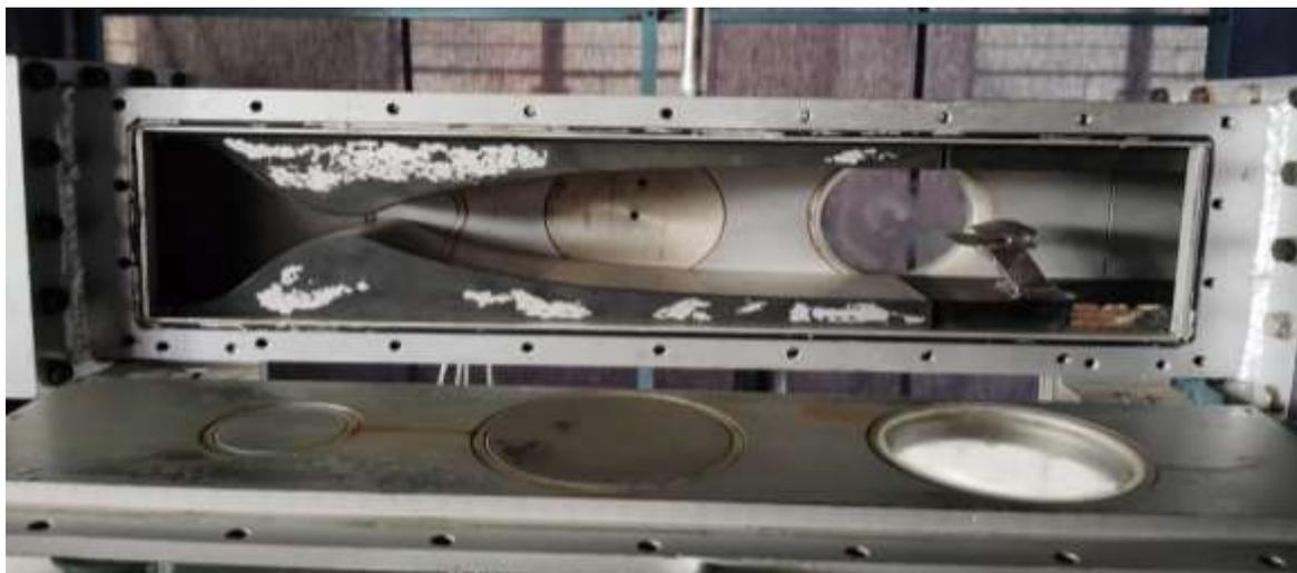
Fig.1.4: Wind tunnel
