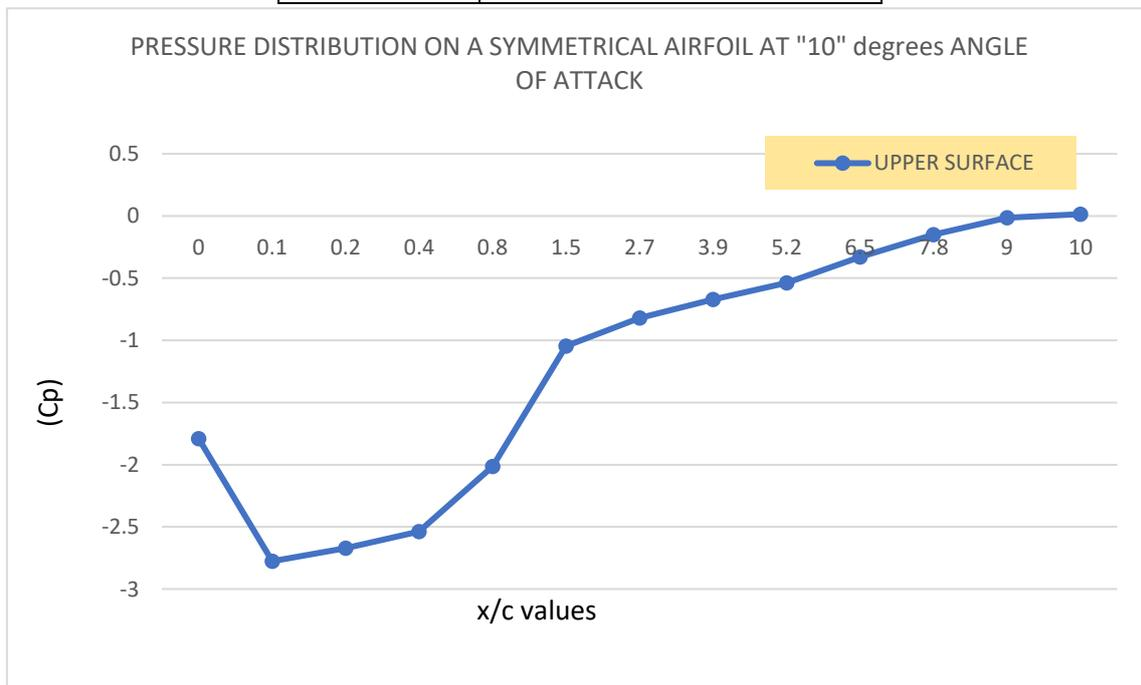
**Fig 6.2:** Pressure Distribution (Cp vs. x/c) graph
