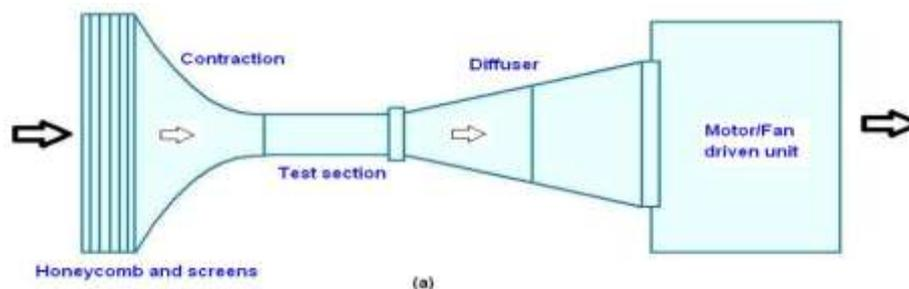
Figure 4.1.1: subsonic wind tunnel test
