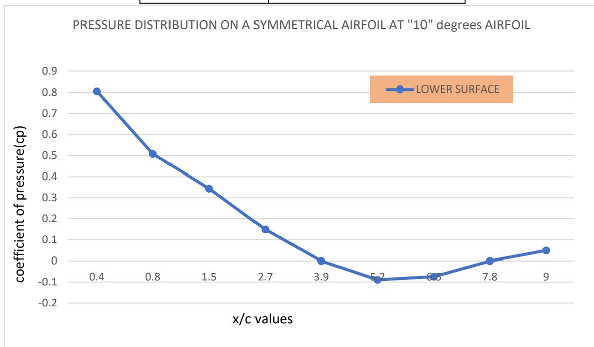
Fig 6.4: Pressure Distribution (Cp vs. x/c) graph
