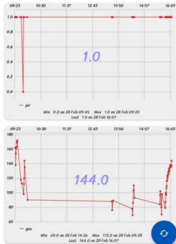
Figure 2C: PIR Motion Detection Data and Gas Concentration Levels Over Time
