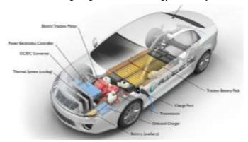
**2.3 Battery Management System (BMS):** The Battery Management System oversees the health and performance of an EV's battery. It monitors charge levels, temperature, and cell balance, ensuring safe operation by preventing overcharging and deep discharging. The BMS optimizes battery life, efficiency, and performance, enhancing overall vehicle reliability.
