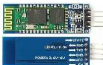
Figure 3.3: HC-06 Bluetooth module
