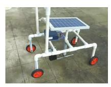
External Frame Work: The external frame work is having 1 inch PVC hallow pipes, elbows and tees. The wheels are attached to the body as shown in fig. the blade is coupled to the shaft of the motor. The motor is attached to the body through the 1 inch by 1.5 inch PVC reduceroverall height of the model is 4.5 ft.
