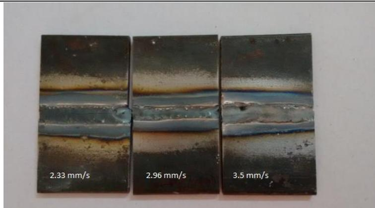
**Fig. 6** TIG welded specimen with TiO<sub>2</sub> flux at 210 A current
