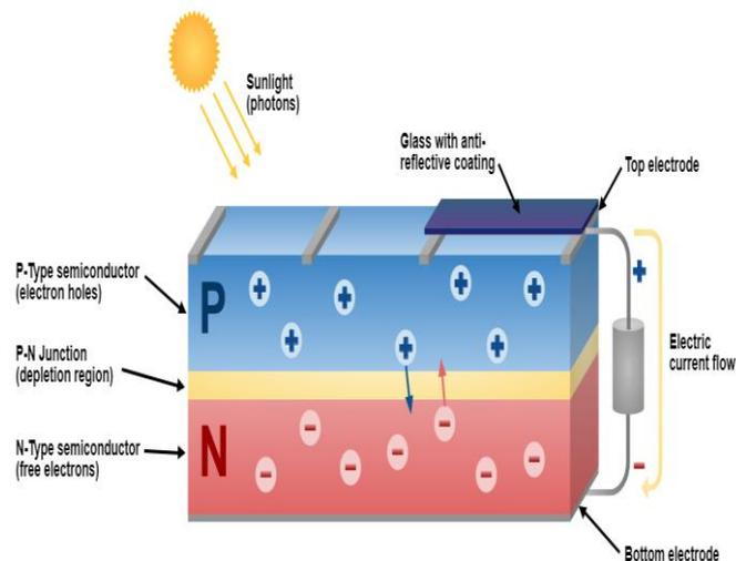
Figure 1 A photovoltaic cell
