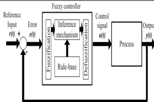
Figure 6 Scheme of a fuzzy logic controller
