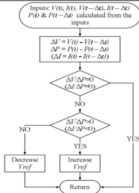
Figure 4 Incremental Conductance
