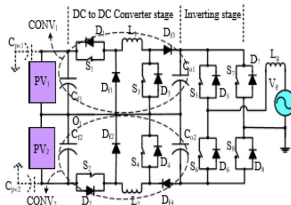
Fig. 5 Dual Buck & Boost based Inverter (DBBI)
