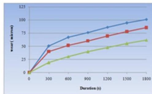
Figure 6.3 Time vs. Wear rate (5N, 1M/S)
