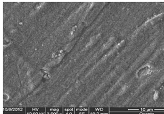
Figure 7.6. SEM micrograph of the worn surface of the Al alloy- 7.5 wt. % composite at a normal load of 25 N with 2.5m/s sliding velocity
