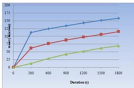
Figure 6.2 Time vs. Wear rate (5N, 2.5M/S)
