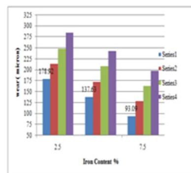
Figure 6.7 Iron content% vs. wear (5N, 2.5M/S)
