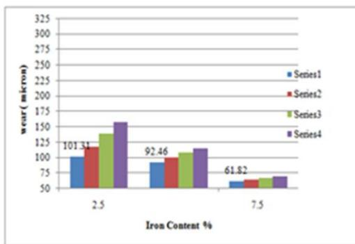
Figure 6.6. Iron content% vs. wear (5N, 1M/S)
