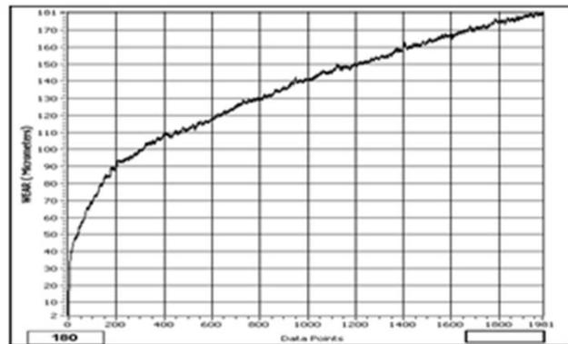
Figure 7.4 Typical curve of wear of Al-5 wt. % Iron oxide composite against steel as a function of sliding velocity at 2 m/s and load 15 N.
